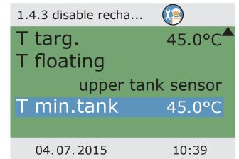
Enter the minimum tank temperature via >T min tank<.
