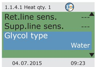
the return line sensor and the supply line sensor must be specified.
