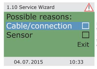
For this malfunction, the following causes are assumed: >Cable/connection< or >Sensor< select the first menu item and confirm by pressing >OK<.
