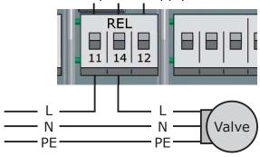
Connection diagram for a switching valve with power supply to REL:
