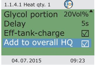
Specify the portion of antifreeze in the exchanger medium as well as the delay.
