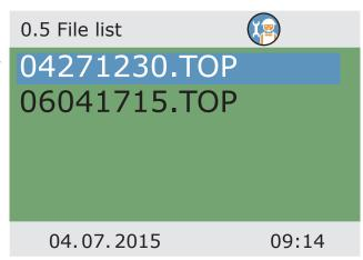
The plant configuration can be saved on the SD card during professional mode operation in the menu "1.2 Settings" by selecting the menu item "Save parameter".
