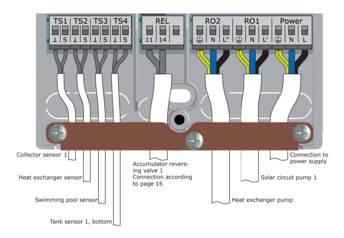
The functions for boiler control are accomplished via the potential-free relay contact which is connected accordingly to the relevant interface of the heating boiler.
