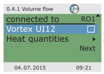
The Vortex sensors for the input of volume flow are selected here.
