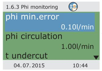
Here, the parameters for volume flow monitoring are defined.
