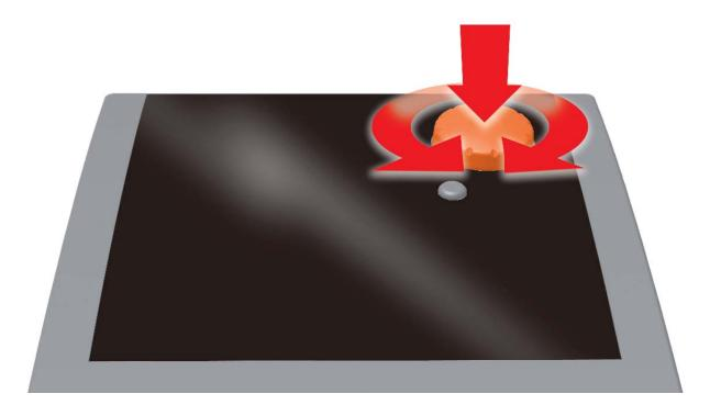
Press the esc button to make the menu return by one level from any subitem.
