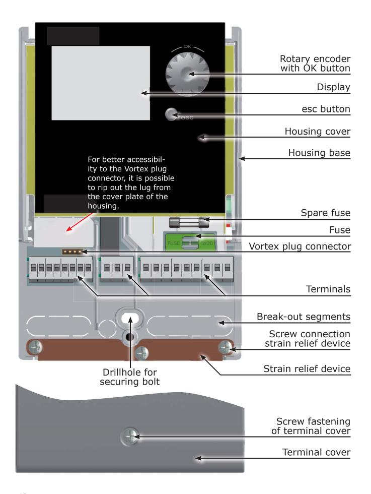
The entire set-up and operation of the differential temperature controller **smart Sol** is effected via only two control elements on the device front.
