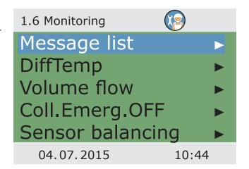
>dT monitoring< is used to define the criteria which lead to fault detection.
