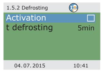
>Defrosting< can be used to heat frozen collectors.
