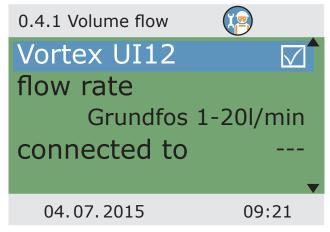
The following variables are provided for volume flow: Grundfos 1-12l/min / Grundfos 1-20l/min / Grundfos 2-40l/min / Grundfos 5-100l/min / Grundfos 10-200l/min / Grundfos 20-400l/min
