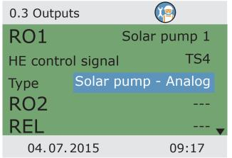
The HE control signal is specified as: analogue solar pump / PWM solar pump / analogue heating pump / PWM heating pump / Wilo ST25/7 PWM.
