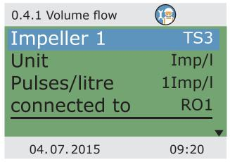
$\dots$  specify the unit as Imp/l or l/Imp as well as the corresponding factor with 1 to 100 Imp/l or 0.1 to 10.0 l/Imp. Select the corresponding output.
