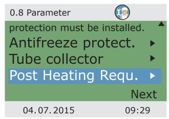
If a hydraulic scheme including boiler control functions has been selected, the post heating requirements are configured here.
