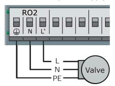
Connection diagram for a switching valve with power supply to RO2:
