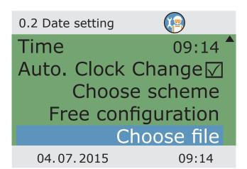
A list of pre-configured plant settings is displayed. Select the desired file and acknowledge with "OK".
