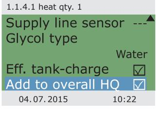
>Add to overall HQ< adds each heat quantity to the overall counter.
