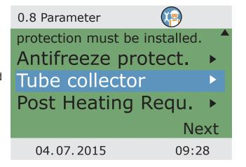
To receive correct measured values from the tube collector system, the pump must be switched ON briefly.
