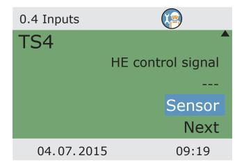
If the volume flow is measured with an impeller, "Impeller 1" must be selected.
