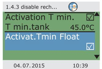
Select the minimum temperature via >T min.tank<.
