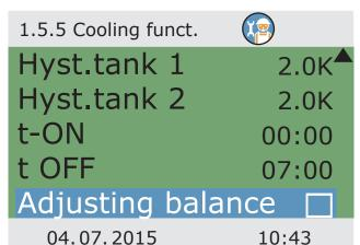
If the adjusting balance is activated, the heat dissipated via the collector is deducted from the energy balance calculation.
