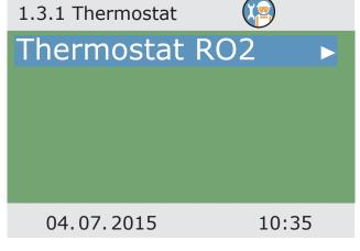
Any controller outputs which are not assigned can be configured as a thermostat.
