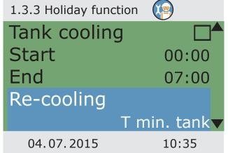
If tank cooling is activated, an appropriate time frame must be defined - this makes sense during the cooler hours of the night - by allowing the controller to dissipate as much energy as possible via the collectors.
